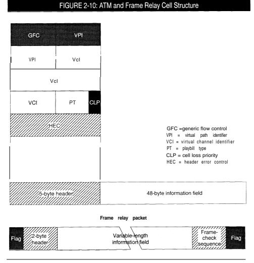
Key' GFC=generic flow control, VPI=vIrtual path identifier, VCI=virtual channel identifier; PT=playbill type, CLP=cell loss priorly, HEC=header error control
