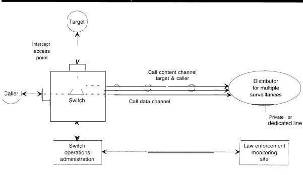
FIGURE 2-5: Generalized Configuration and Functional Components for Electronic Intercepts at a Service Provider's Switch
