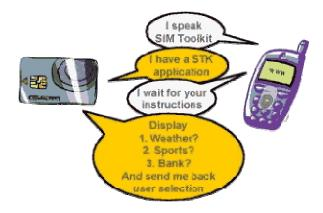
Figure 17 – Communication between the phone and the SIM  $^{\rm 13}$
