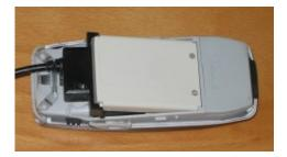
Figure 8 – Nokia 3310 with F-BUS cable attached
