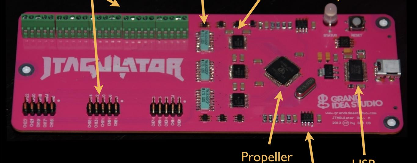
\*\*\* 2x5 headers compatible w/ Bus Pirate probes, http://dangerousprototypes.com/docs/Bus\_Pirate
