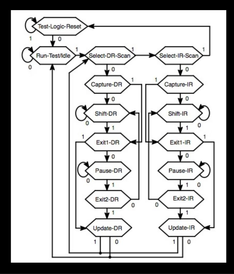
\*\*\* State transitions occur on rising edge of TCK based on current state and value of TMS
