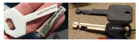
Figure: A 3D printed car key, by Ryan Weaving, and a 3D printed disc detainer key, by Nirav Patel.
