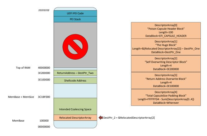
Figure 6: DescriptorArray[1] abuses the CopyMem optimization trick and IsOverlapped integer overflow to wrap DestPtr around the address space.
