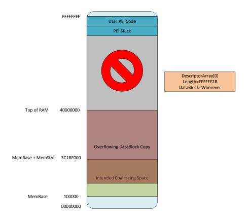
Figure 4: First Attempt at Coelescing Exploitation fails due to the address space gap
