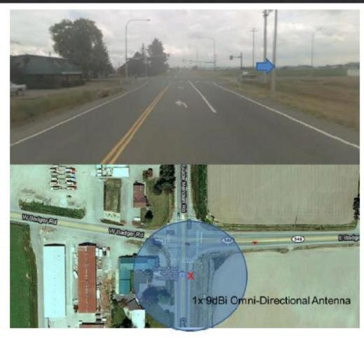
Figure 4-5: SR 539 and Badger Rd. Bluetooth installation location
