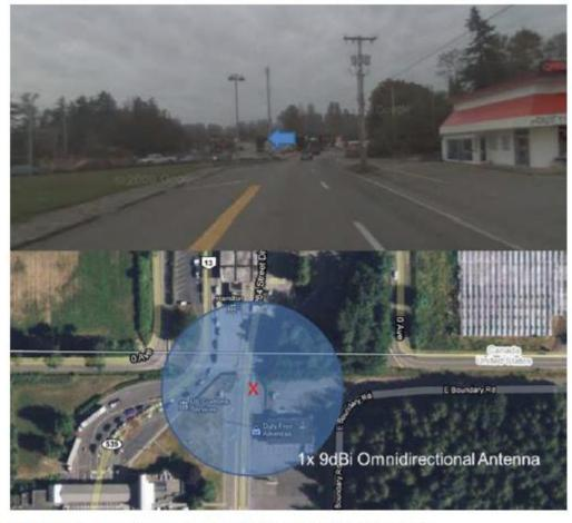
Figure 4-6: SR 539 U.S.-Canada border Bluetooth installation location
